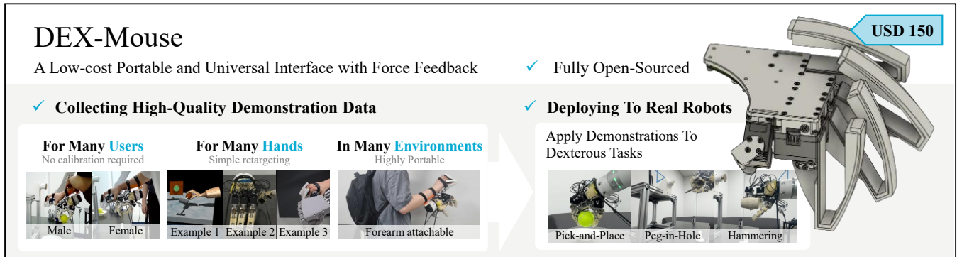
Fig. 1: An overview of DEX-Mouse. The proposed USD 150, fully open-sourced teleoperation interface enables scalable collection of high-quality demonstration data. Its calibration-free and highly portable design seamlessly accommodates diverse operators, various target robot hands, and diverse real-world environments. Furthermore, collected demonstrations can be directly deployed to diverse dexterous manipulation tasks.
